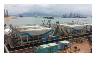
high pressure pumps with four-inch pistons were used to install the large-diameter grout columns and a single Soilmec 7T-505 pump was used for the small-diameter columns.
